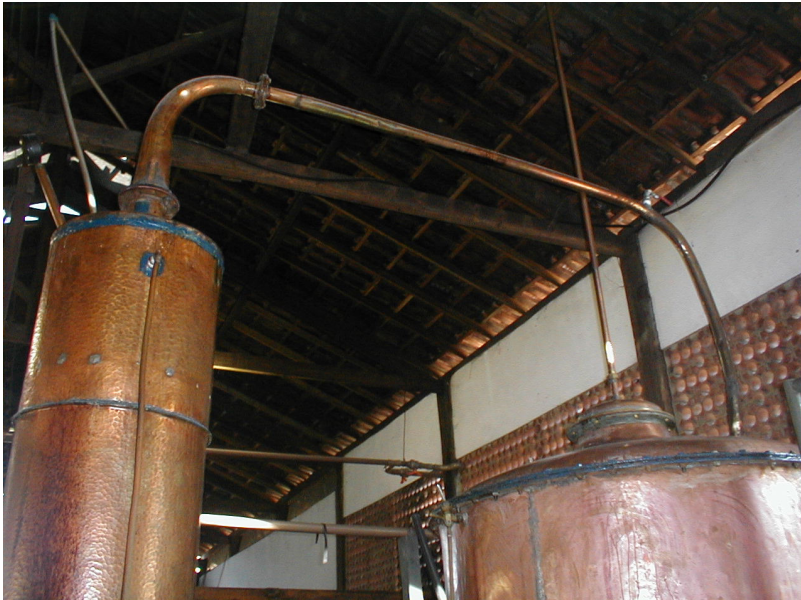
Fig. 11. Column (at the left) with temperature control by a tubular dephlegmator (alembic JLG ; Bemposta-RJ).
