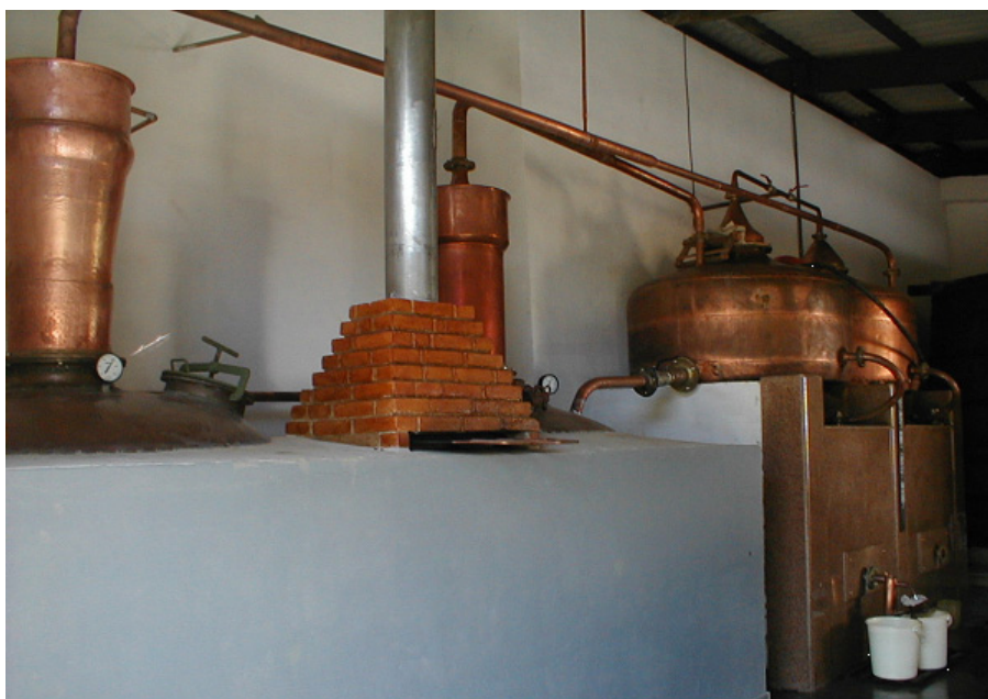
Fig. 2. Two two-body alembics with direct heating (CQE A and CQE B, Paraty-RJ)
