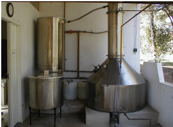
Fig. 14. Alembic with stainless steel pan and serpentine coil (Resende-RJ).
